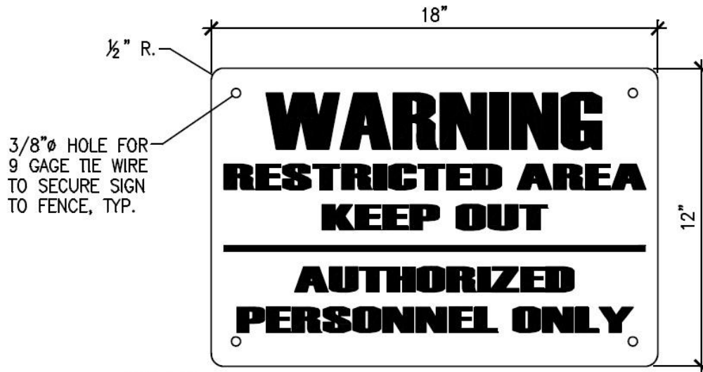
Figure 4-6: Warning Sign "B"
